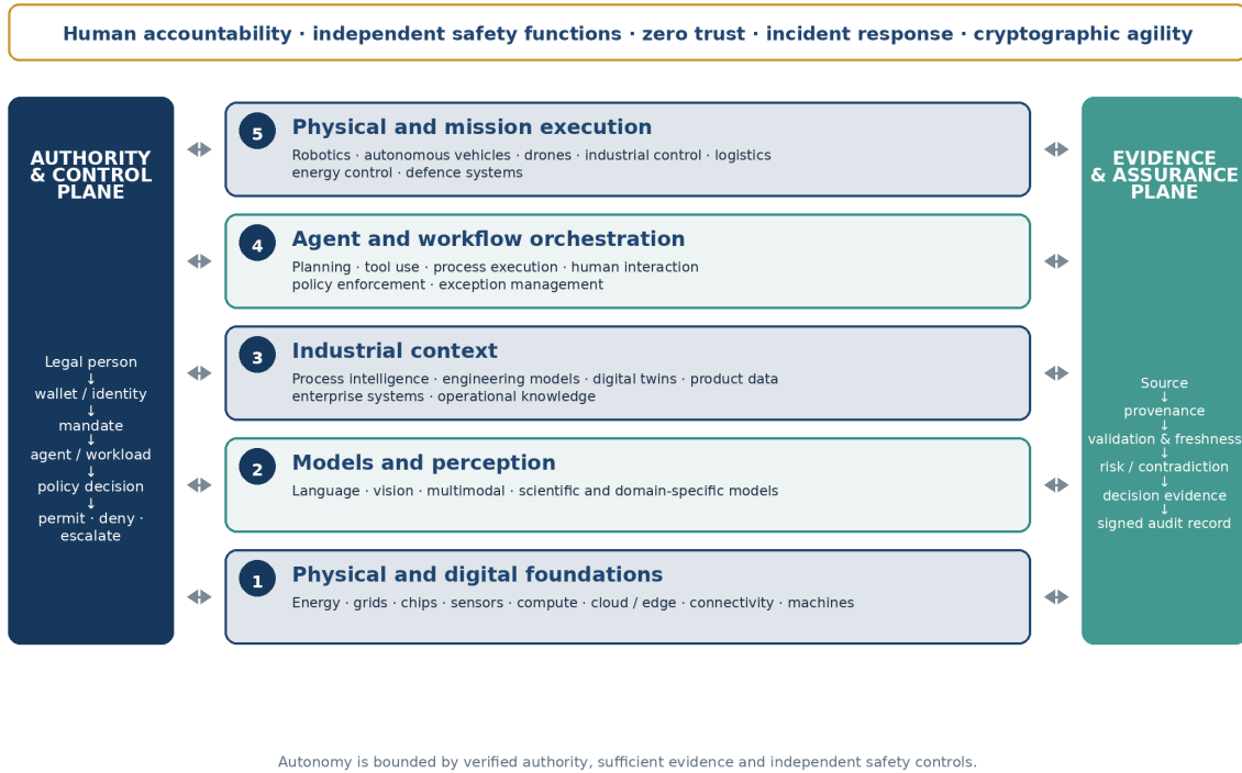
Figure 4: Reference architecture for agentic cyber-physical systems. Source: author’s conceptual synthesis.
